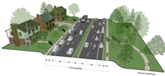
Existing Typical Section (Segment 1)
