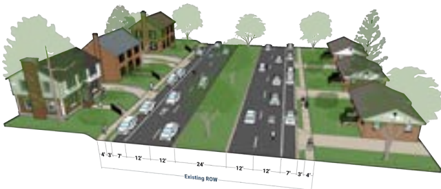
Existing Typical Section (Segment 3)
