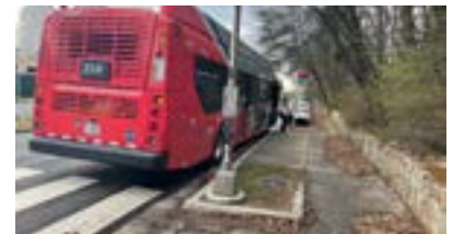
Curb extensions at bus stops (e.g. at National Guard Bureau Pedestrian Hybrid Beacon) shorten crossing distances.
